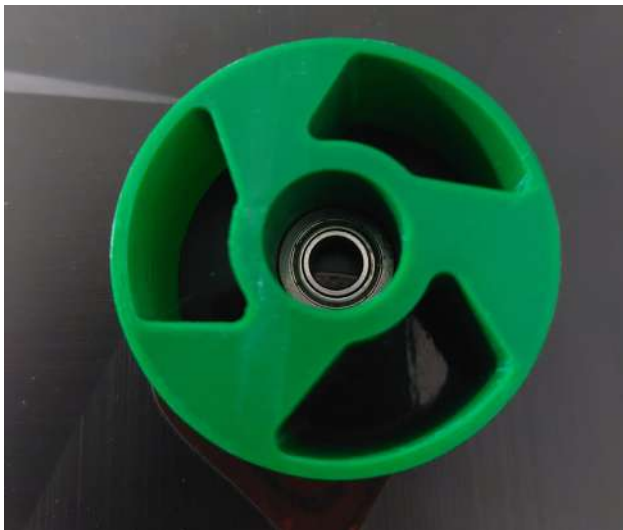
Dead Wheel nou, printat 3D cu rulment integrat
