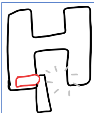
The motor is drawn in red, and the dotted grey space is where the hanging arm should fit
